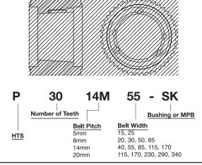
"P" HTS Sprockets (RPP Tooth Profile) – Runs with RPP, RPP+, Hawk Pd<sup>®</sup>, & HTD<sup>®</sup> belts.
